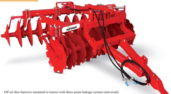
Off set disc harrows mounted to tractor with three point linkage system (universal) and trailed by drawbar. Machine can be easily transported to field. These disc harrows are used for chopping of stems and mixing with soil after harvesting. After using of plough, chisel and cultivators on the field, you can use this disc harrow for breaking of clods and crumbling of soils.
