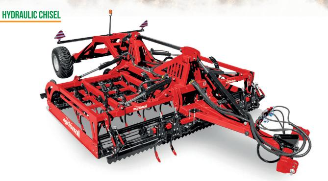
The machine has powerful tines working down to 30-40-45-50-55-60 cm depths. You benefit from a spacious frame construction offering impressive mixing capabilities. It is the ideal tine tiller for those looking for high quality working results, performance and durability.
