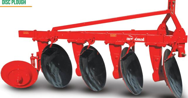
Disc Plougs can be produce with 2-3-4-5-6 and 7-8-9-10 discs. It is working easily At stony, rocky and tree roots covered terrains. On Profile chassis owning ploughs is possible to remove the body. Point of structure and construction producing is standard. Disc plough discs are making (way angle) the direction of movement coplanar and according the soil surface (status angle) is making a angle.
